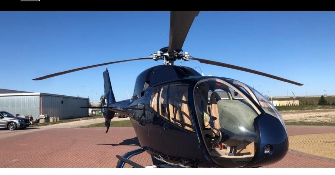
Single-engine, light utility helicopter, designed and developed by Eurocopter.
